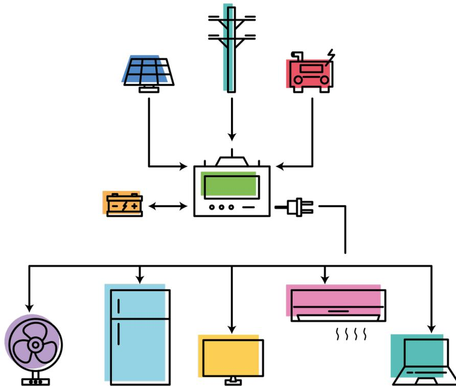
FIGURE 1: PV SYSTEM WITH HYBRID INVERTER
